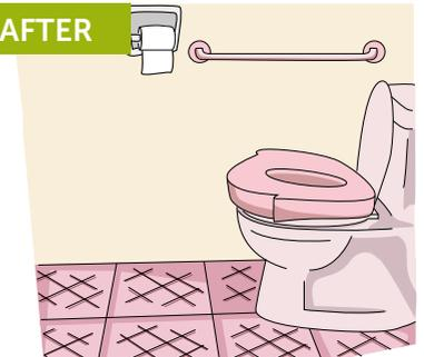
A sitting toilet with an additional toilet raiser, installation of grab bar and anti-slip floor treatment
