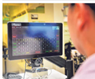
EyeGate Edge has a camera that monitors the user's eye movements to determine where he is looking on the screen. ST PHOTO ALPHONSEUS CHEIN
