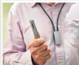
The Roger Pen microphone amplifies audio and sends it to the user's hearing aid. In the background is the Roger MyLink receiver. ST PHOTO ALPHONSEUS CHEIN
