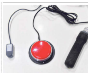
Adaptive switches that are actuated by being (from left) tapped on, pressed and squeezed. ST PHOTO ALPHONSEUS CHEIN
